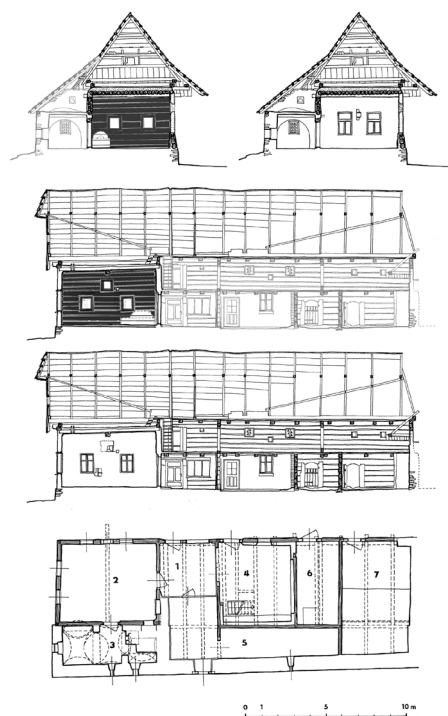
Figure 5. Čistá u Litomyšle, distr. Svitavy, farmhouse No. 171 with „smoky” room dated 1583; the restitution of the „smoky” room and the current state with the „light” room; 1 - entrance hall, 2 - living (all purpose) room, 3 - kitchen / chamber, 4 - chamber—granary, 5 - descent to the cellar, 6/7 - stables?. (Credits: Jiří Syrový).
